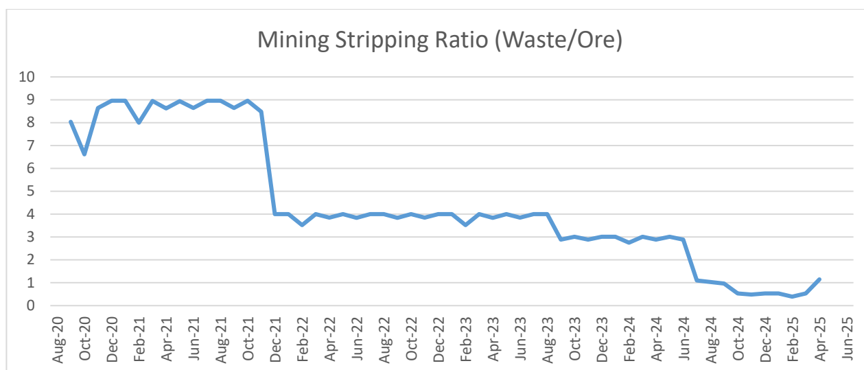
Figure 3-8: Forecast mining stripping ratio
